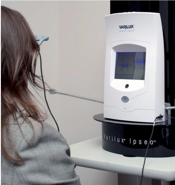
Figure 20-24. The VisionPrint System is used to measure head and eye movements. Results determine how the Varilux Ipseo personalized progressive lens will be custom designed for the head and eye movement requirements of the wearer.
