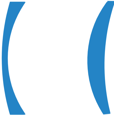
Figure 12-49. A meniscus lens has a plus (convex) surface on the front and a concave (minus) surface on the back.
