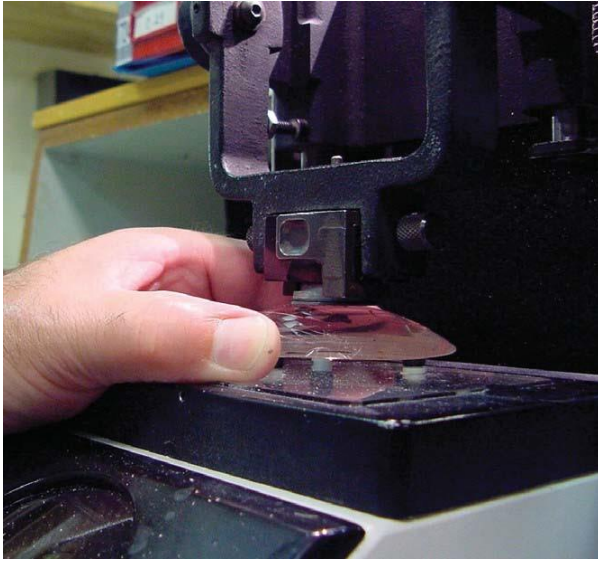
Figure 24-13. The lens is being blocked for edging.
