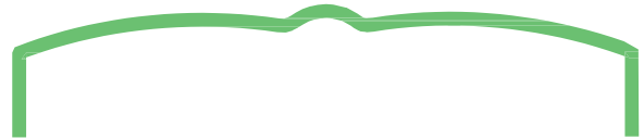
Figure 23-5. The high mass impact test drops a pointed, 1- inch diameter projectile onto safety eyeglass frames from 51.2 inches to test their suitability for use as Z87 safety frames.
