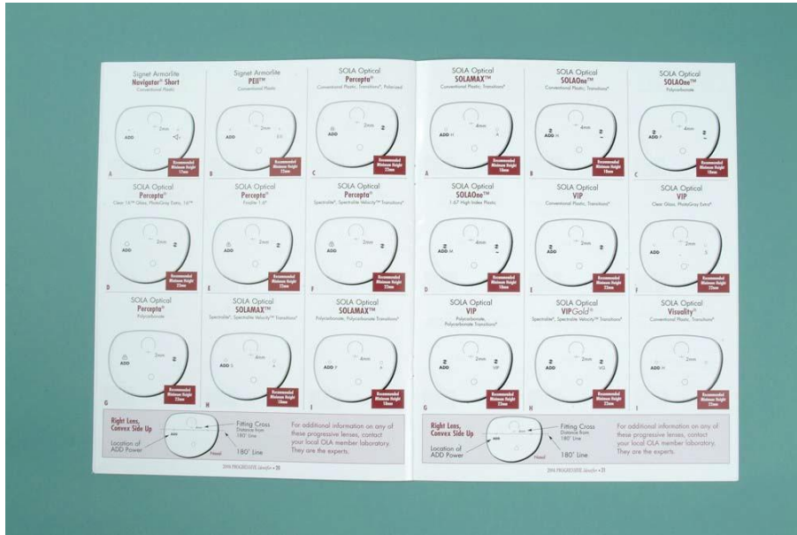
Figure 20-15. This is a page from the Optical Laboratory Association's (OLA) Progressive Identifier used to find information about progressive addition lenses.
