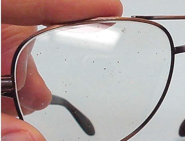
Figure 23-1. Welding or grinding spatter will pit or permanently stick to glass lenses, as shown here. It does not adhere to plastic lens material.
